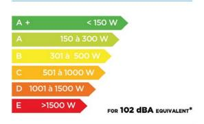
\*The figure given represents the electrical power dissipated by the speaker to generate over its bandwidth a sound level equivalent to 102 dBA with a pink noise input. For calculation purposes, the speaker is considered being part of an equalized sysytem with absolutely flat response from 20 Hz to 20 kHz.
