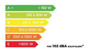
\*The figure given represents the electrical power dissipated by the speaker to generate over its bandwidth a sound level equivalent to 102 dBA with a pink noise input. For calculation purposes, the speaker is considered being part of an equalized sysytem with absolutely flat response from 20 Hz to 20 kHz.
