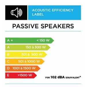
\*The figure given represents the electrical power dissipated by the speaker to generate over its bandwidth a sound level equivalent to 102 dBA with a pink noise input. For calculation purposes, the speaker is considered being part of an equalized sysytem with absolutely flat response from 20 Hz to 20 kHz.
