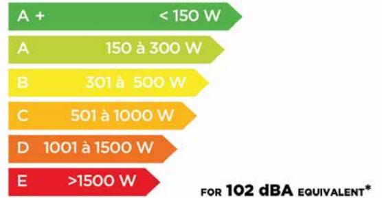
\*The figure given represents the electrical power dissipated by the speaker to generate over its bandwidth a sound level equivalent to 102 dBA with a pink noise input. For calculation purposes, the speaker is considered being part of an equalized system with absolutely flat response from 20 Hz to 20 kHz.
